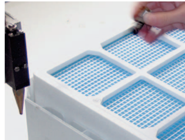
Filter quality control of a HyperHEPA® filter
